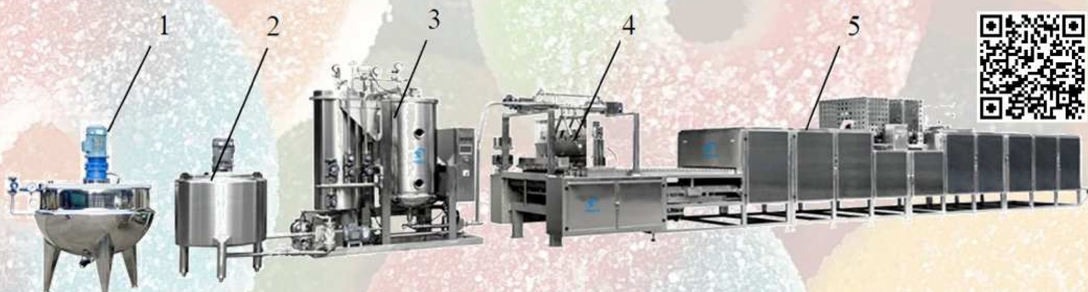
Figure 1. Jelly candy production line by Ningbo Youlu Machinery Technology Co: 1-system of automatic weighing and dissolution of components; 2-a storage capacity; 3-a vacuum cooking boiler; 4-a depositing machine; 5-a cooling tunnel.
