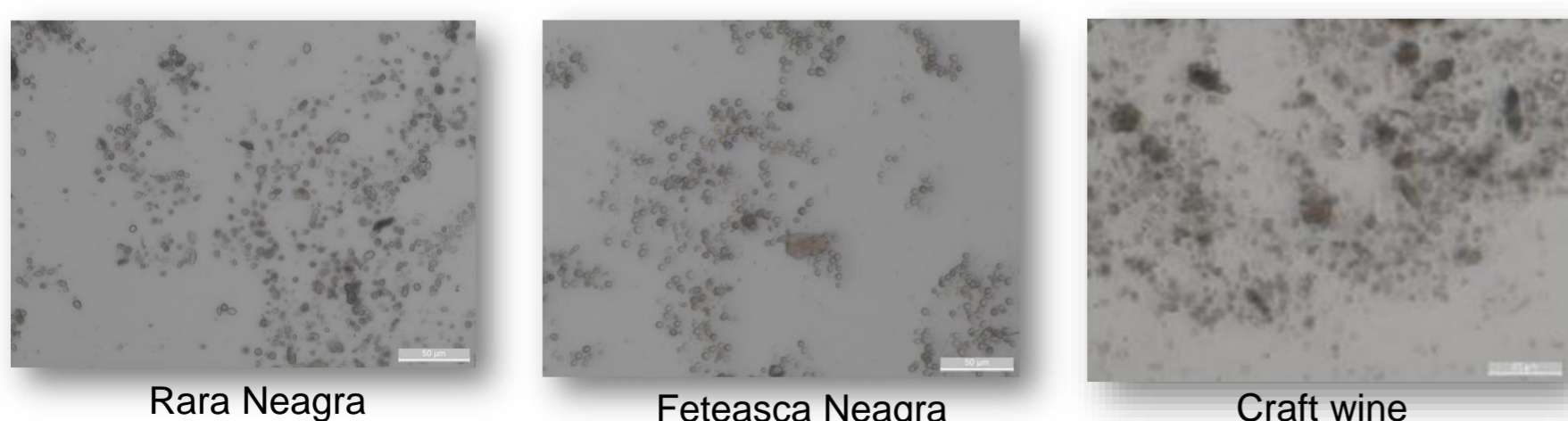
Microscopy of suspensions with added beta-glucans: The average size of microparticles after sonication is 3-4 µm
